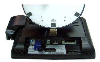
• Connect one end of the **video cable** to the rear side of computer and the other to the LCD monitor. Tighten by turning the two thumb screws clockwise to ensure proper grounding.
